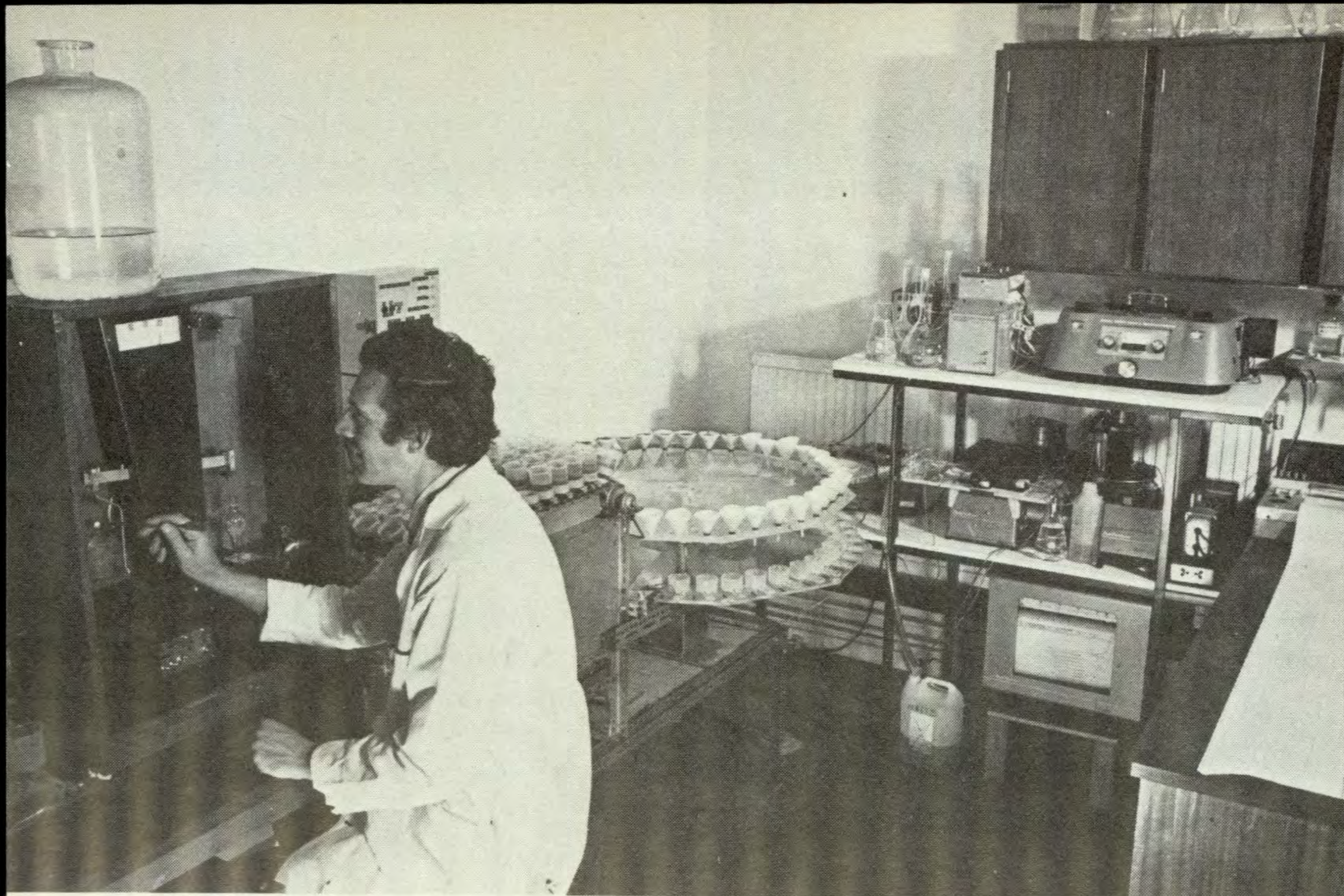
Fig. 1. Sample preparation unit developed at WRO, linked to double channel auto-analyser.
