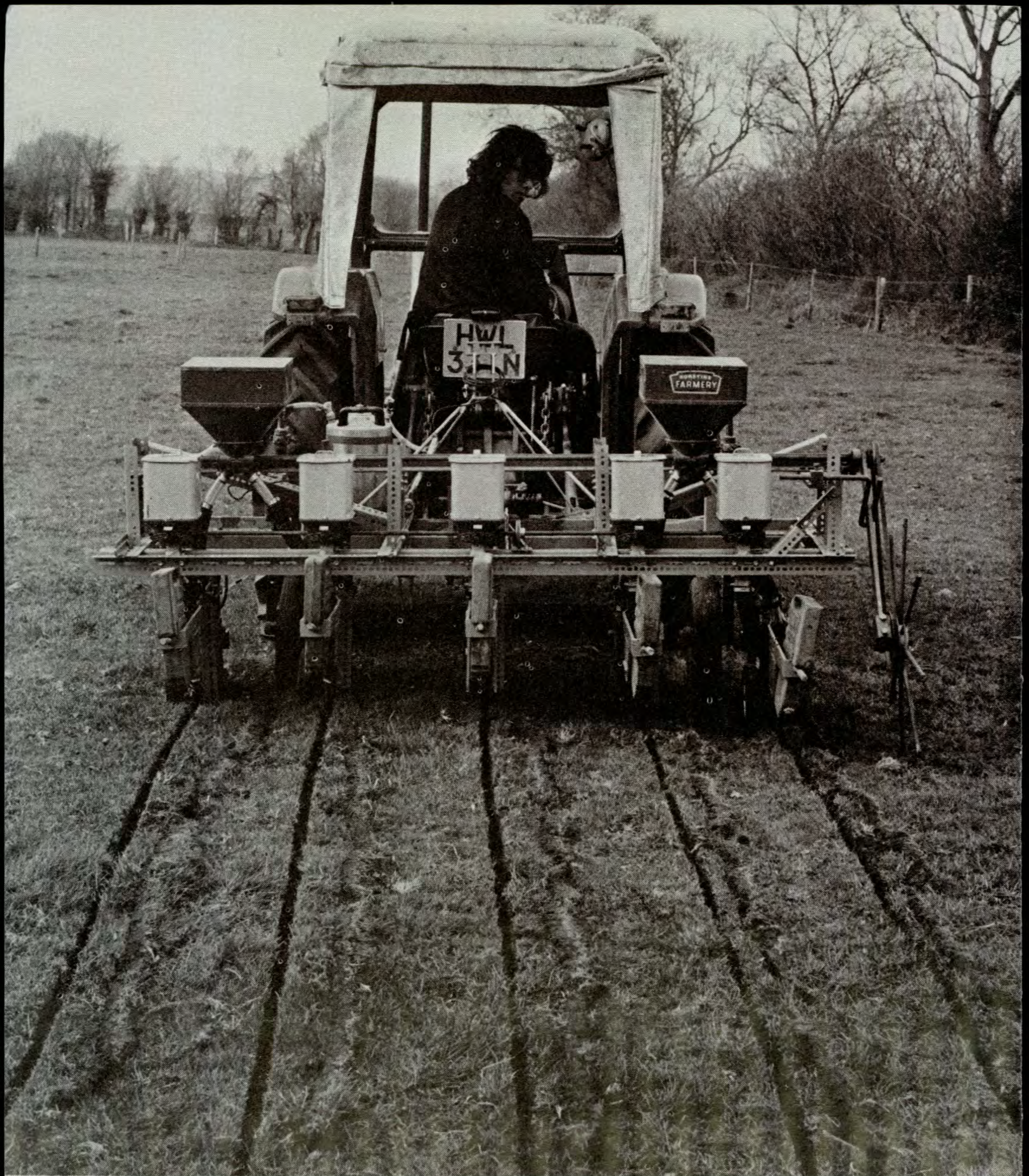
This 5-row tool frame assembly of components has been used to develop the WRO technique of one-pass re-seeding of old pasture. Each unit simultaneously applies a narrow band of growth-suppressing herbicide, removes a strip of turf down the centre of the band leaving a slot 2-3 cm wide and deep, into which is sown seed, fertilizer and slug pellets. (See article on p. 68).
