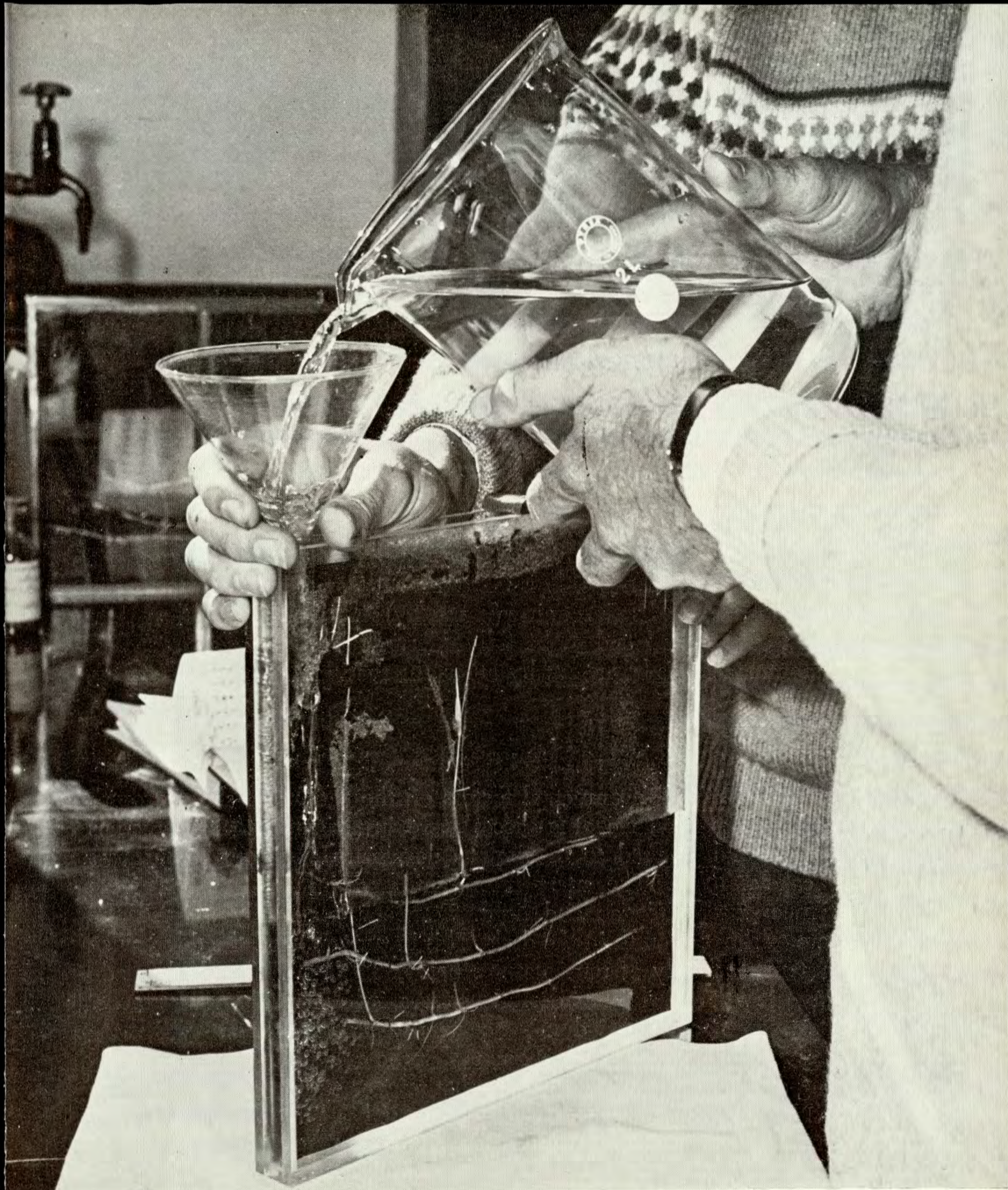
Using the small perspex growth chambers illustrated here, the growth of buds and shoots on couch rhizomes can be studied without disturbing them.
