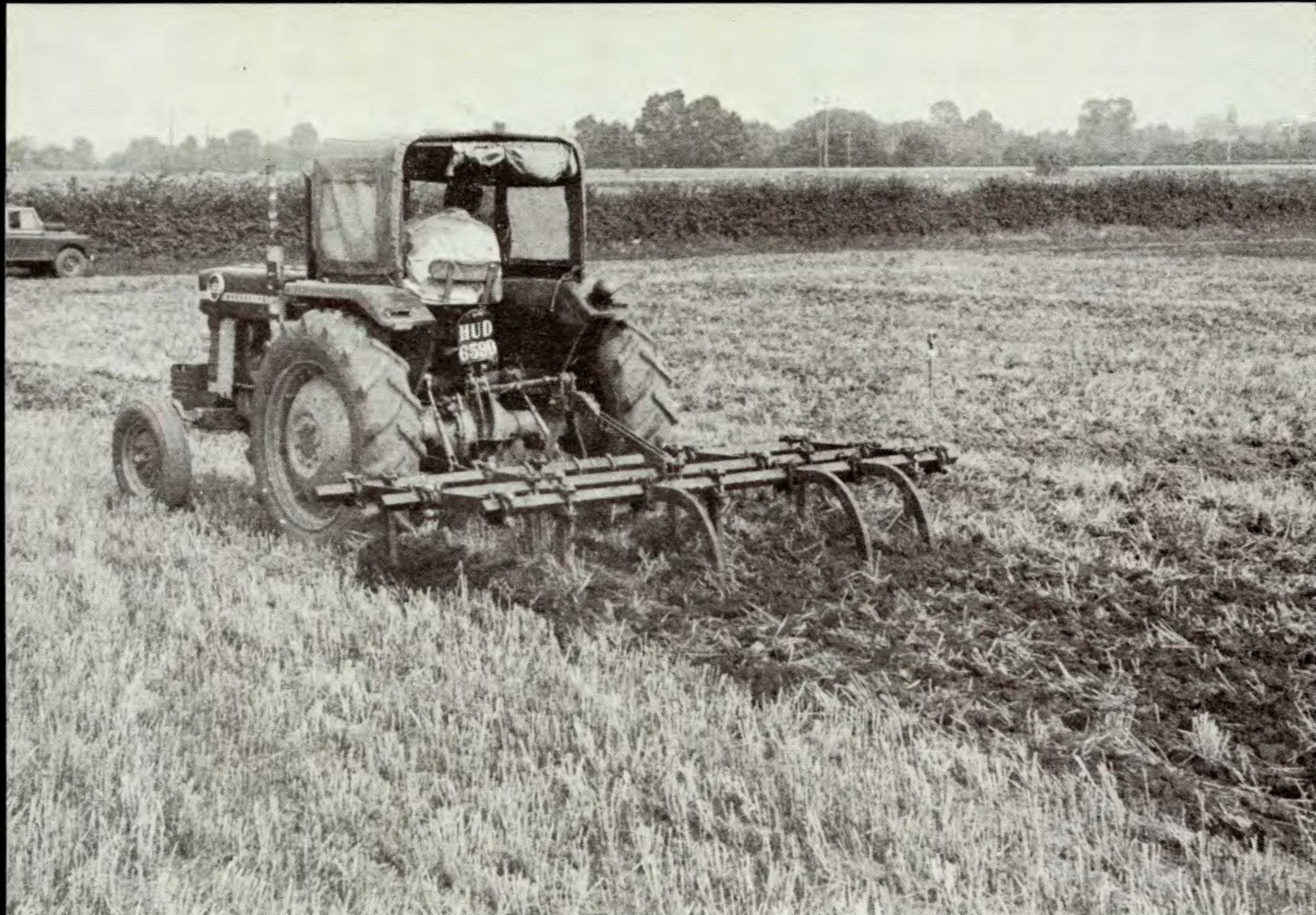
Post-harvest cultivation of cereal stubble for couch control at WRO. The aim is to fragment the rhizomes to stimulate dormant buds into active growth, rendering them vulnerable to subsequent cultivations or sprays.
