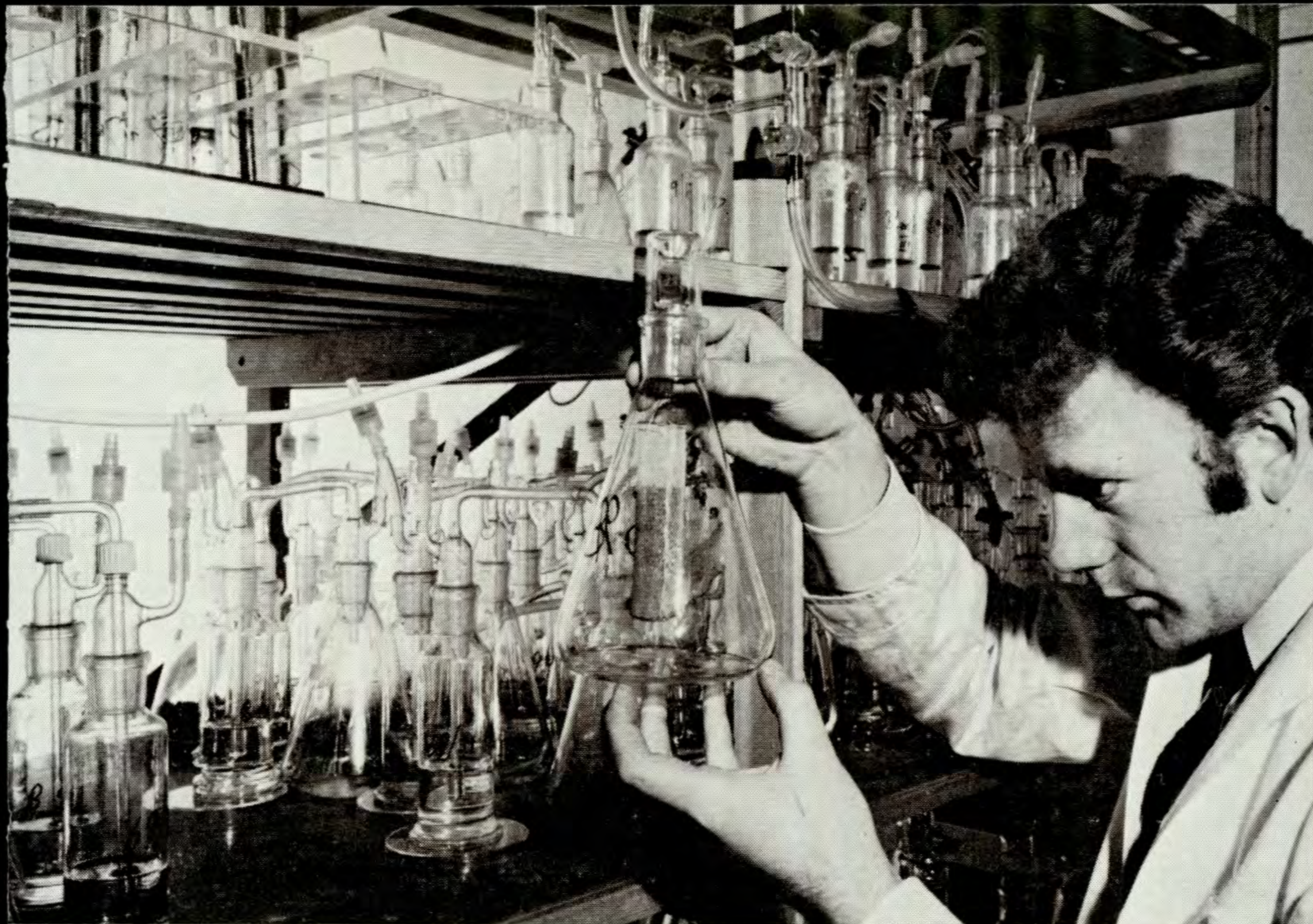
A Ph.D. student, attached to WRO, setting up an experiment to measure the effect of different herbicides on the respiratory \text{CO}_2 production of soil micro-organisms.
