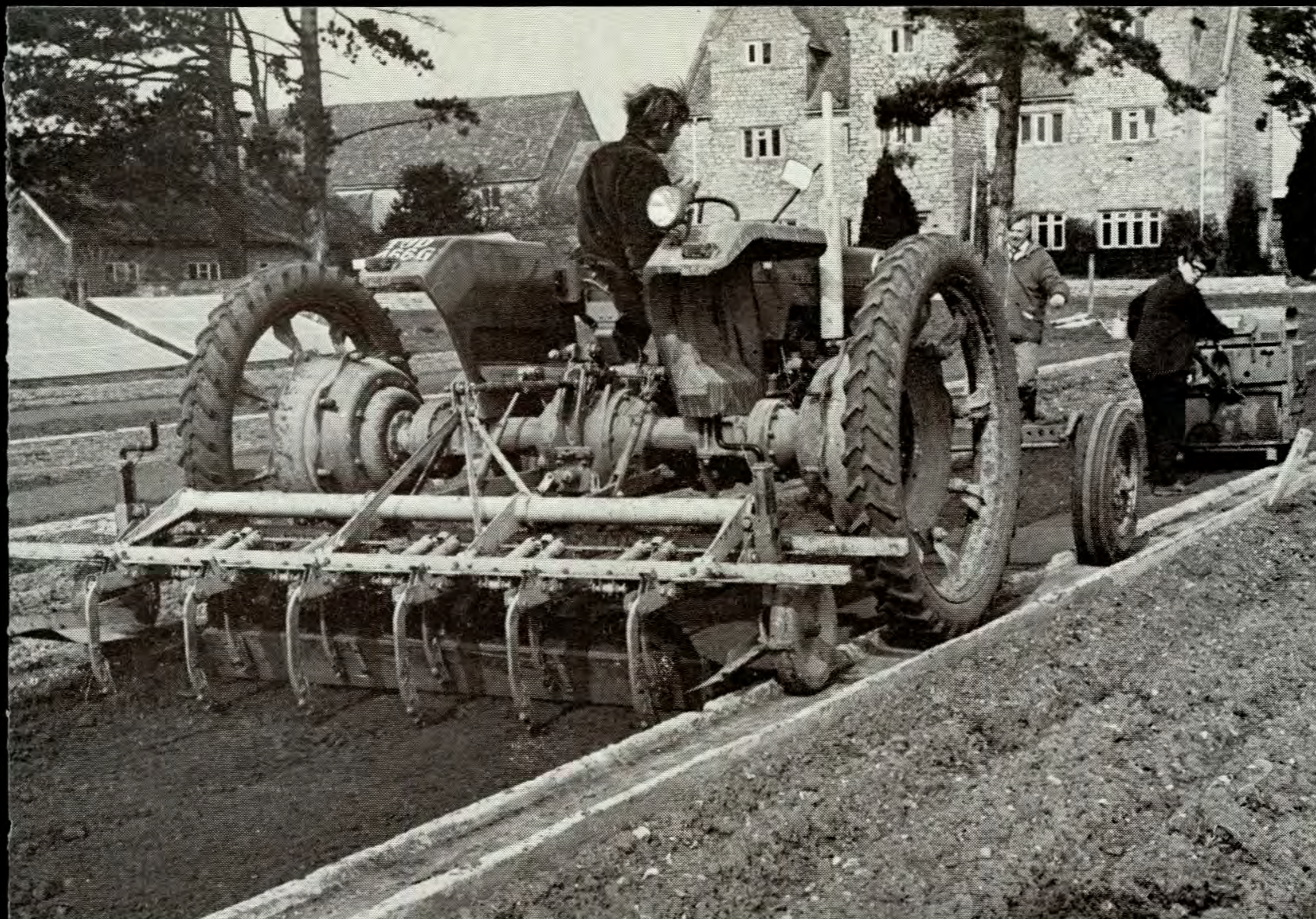
Tillage investigations without 'wheelmarks'. This experimental site at Begbroke is provided with concrete 'tracks' to avoid the soil compaction caused by tractor wheels and enable accurate control of implement penetration.
