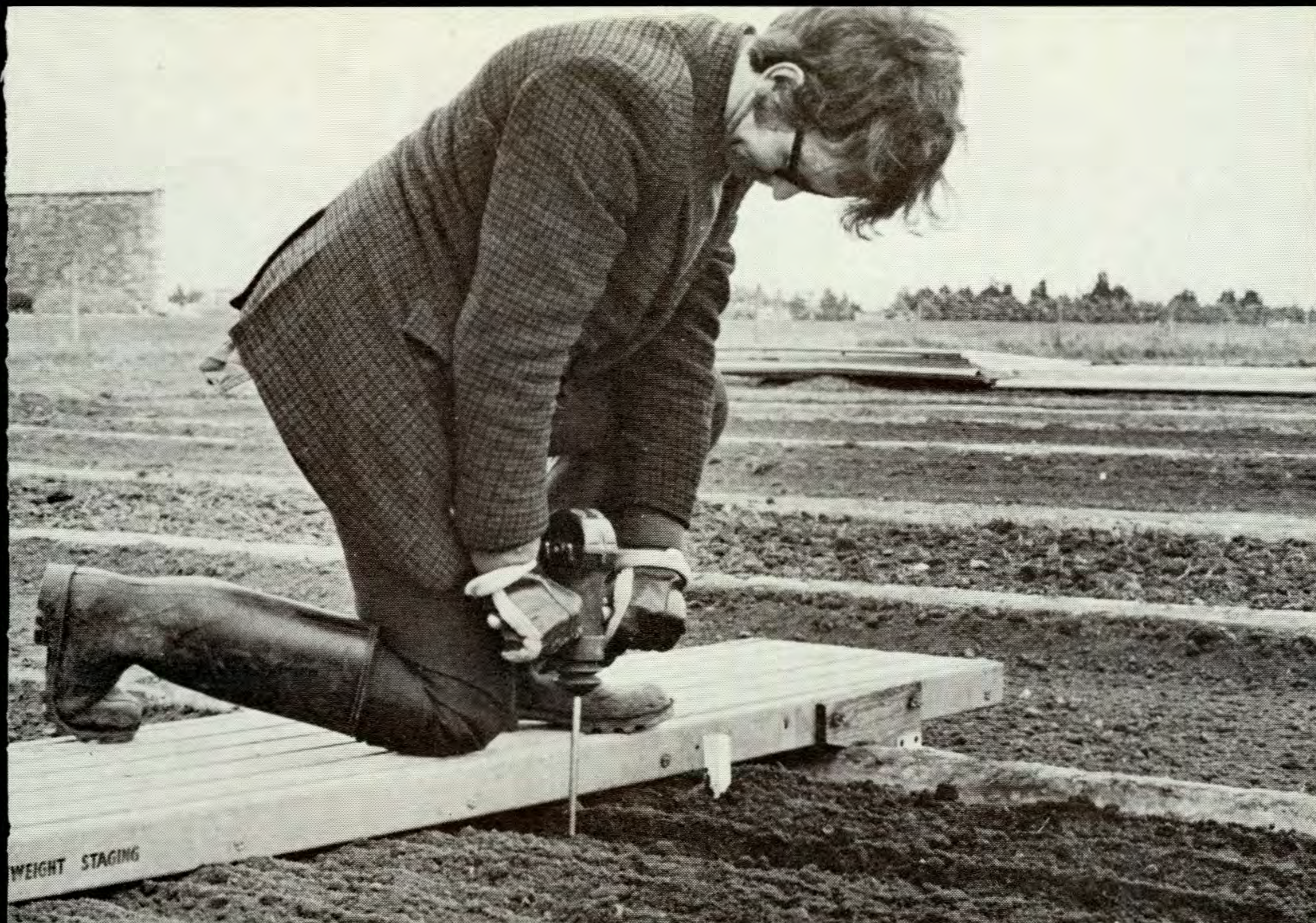
A Letcombe Laboratory member of the Joint WRO/Letcombe Cereals Tillage Project assesses the effect of various tillage treatments on soil compaction.
