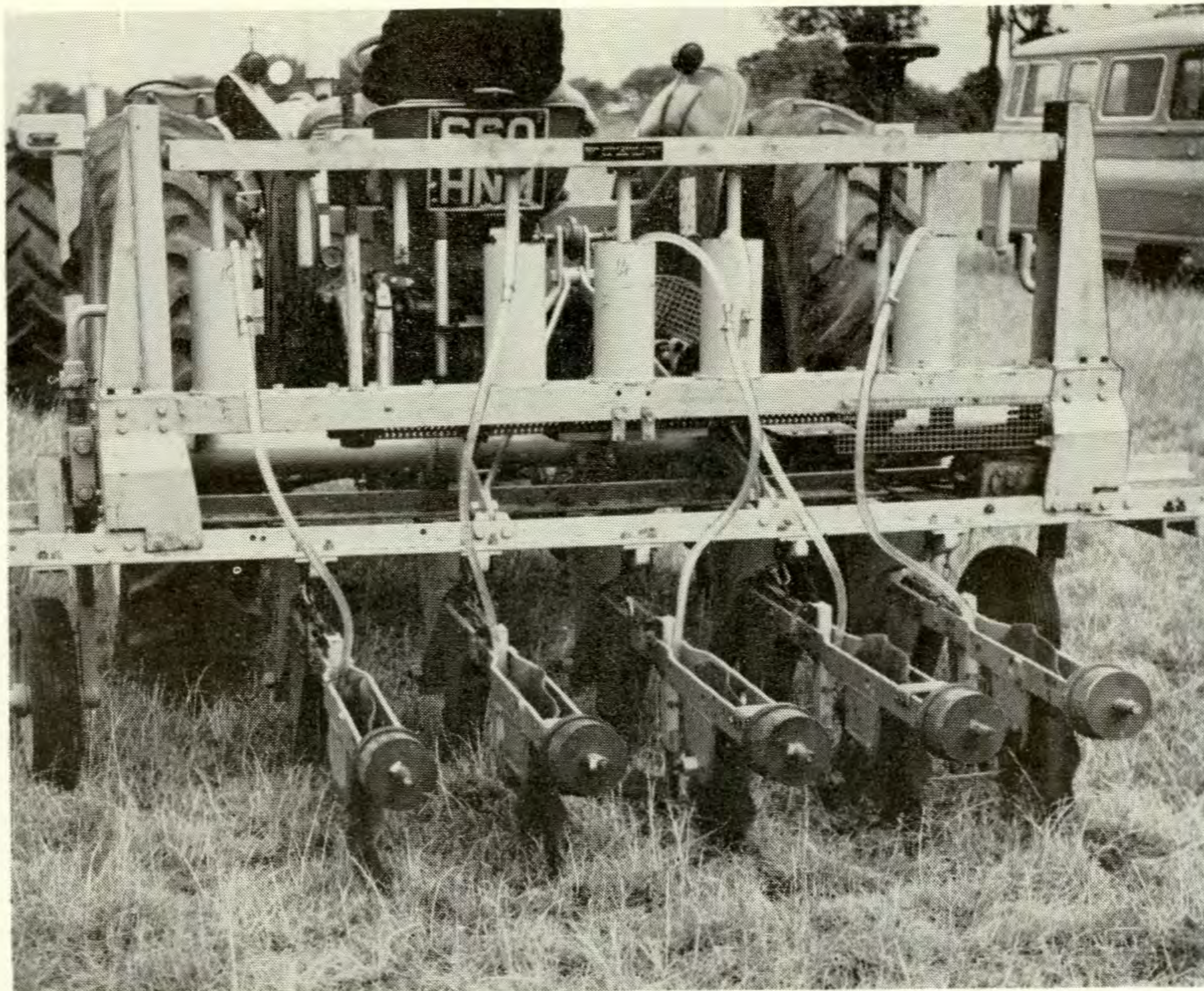
A prototype "fluid drill" for injecting seeds suspended in an aqueous fluid into cultivated or uncultivated soil.
