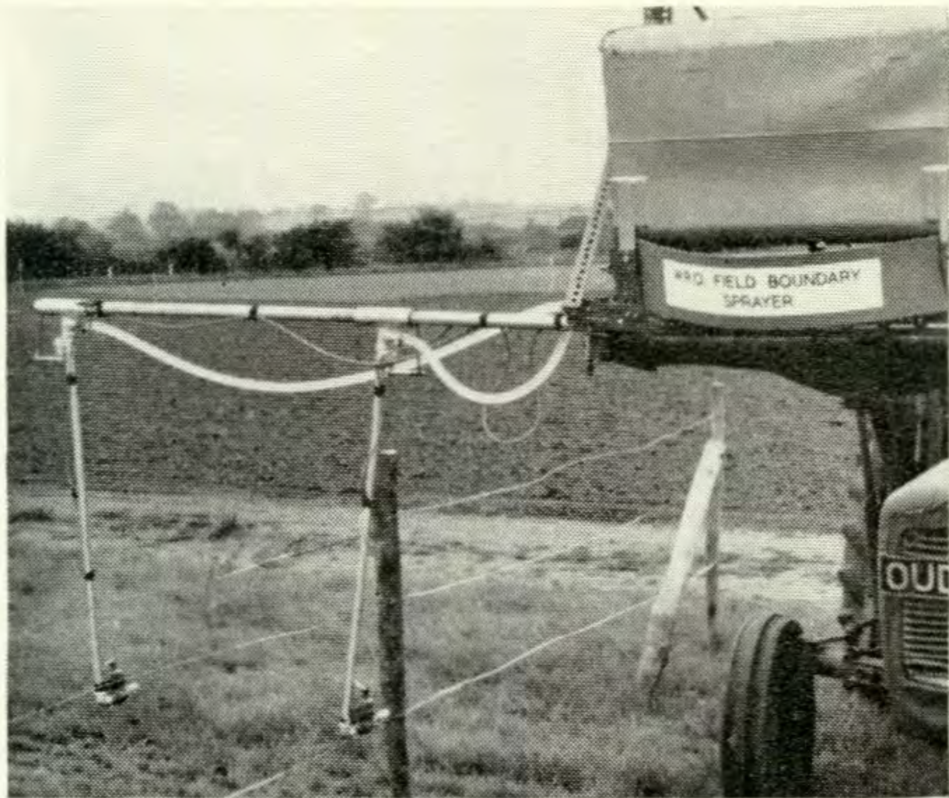
Equipment for spraying fence lines based on two "Vibrajet" drift-free nozzles.
