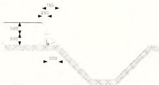
Figure 3. Typical lay-out of a field sprayer above a sugarbeet crop in the Netherlands. When the ditch-bank is 1.5m wide, the distance between the last crop-row and the surface water is 2.0m.
