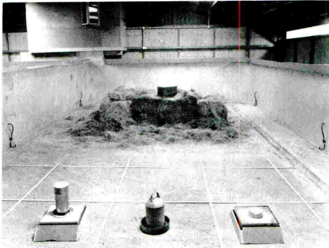
Plate 1. The rat arena: in the foreground are the feeders, novel on the left, familiar on the right, each mounted on an electronic balance, between them is the water font, behind this the stack with the nest boxes and in the background the observation hut.
