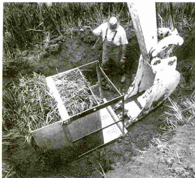
Figure 7: Filling of a lysimeter with an undisturbed soil monolith
