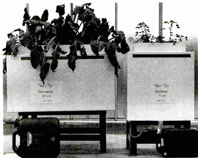
Figure 2: Lysimeters ready for use, filled with soil from the plough layer (left) or an undisturbed soil monolith (right).
