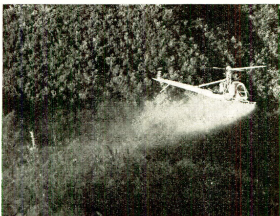
FIG. 1.—Hiller helicopter spraying gorse in New Zealand with 2,4,5-T butyl ester at 3.6 lb. acid equiv. in 60 gal. of water/acre. Application made in four passes over the target, each at 15 gal./acre
