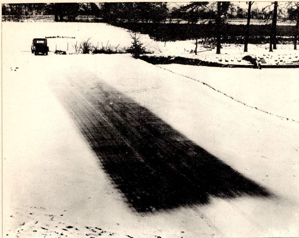
A dye sprayed onto snow showing logarithmic decrease in dosage. Halving of dosage occurs every 6 yards
