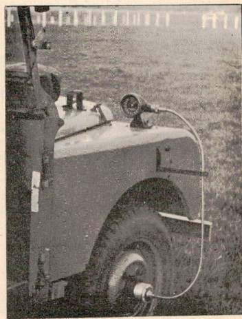
Fig. VI. LAND ROVER SPRAYER FOR LOW VOLUME APPLICATIONS. Showing speedometer and drive for use while spraying.
