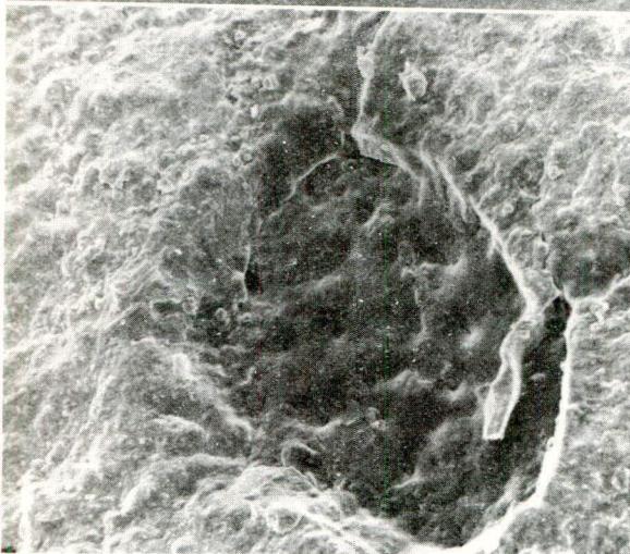
Fig. 3 Scanning electron micrograph showing a section of encapsulation coat removed by an adhering seed. The seeds were treated with Daran 8600.
