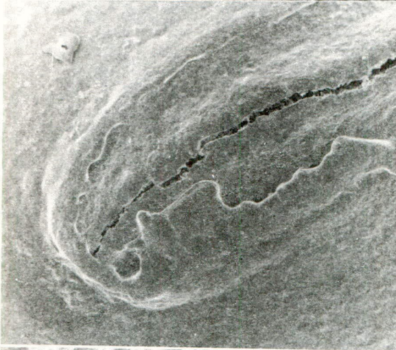
Fig. 2 Scanning electron micrograph of a crack in the encapsulation coat on a soybean seed treated with Daran 8600.
